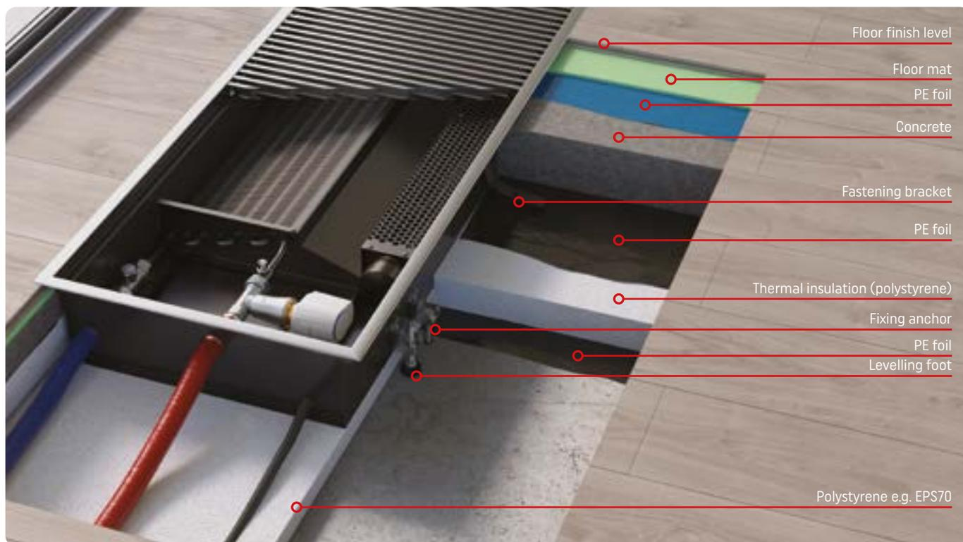
Before starting the assembly, take out and secure the heating kit (fan, airflow targeting sheet and heat exchanger). After that, install assembly struts on the casing edge.
