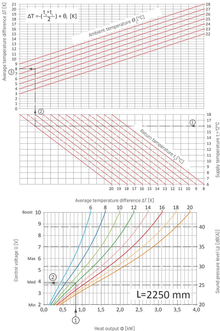
1. Draw a horizontal line starting from the supply temperature (12 °C). End the line on the crossing with return temperature line (16 °C).
