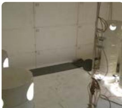
The research of heating and cooling power of CVK trench units was carried out in a specially prepared climatic chamber, in accordance with the requirements of the European Standard EN-16430 in cooperation with the HLK Stuttgart laboratory at the Institut für Gebäudeenergetik Universität Stuttgart.
