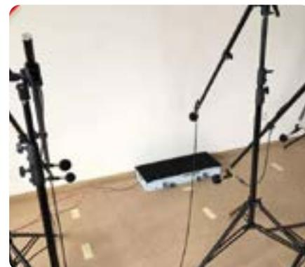
The acoustic power measurement of the CVK series units is carried out in accordance with the European standard EN ISO 3744 at the headquarters of VERANO. The measurement is made at points located on the measuring surface surrounding the tested fan coil over the sound reflecting plane. Thanks to the use of a digital sound analyzer, it is possible to measure broadband as well as in octave bands.
